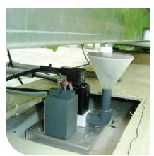
The Priva Root Optimizer calculates the water absorption and determines the optimal water dose based on the substrate weight, the water dose and the quantity of drain water. This ensures that the moisture level of the substrate is always optimal and the crop is able to keep transpiration, growth and the absorption of food in balance.
